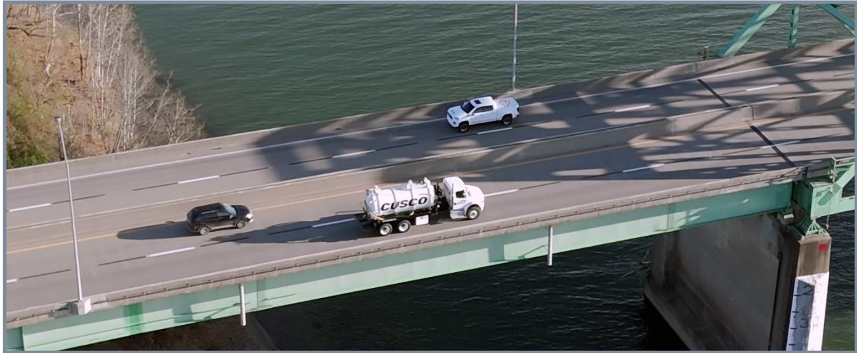
Code tanks are required by the US DOT to be 3rd-party certified for hazardous waste containment during transport. In isolation, this regulation creates a secure holding environment. When placed on a chassis, however, and driven down the road, the potential for collisions and rollovers creates damage risk, especially to valves, manways, and any other tank penetrations, that can result in loss of containment.
